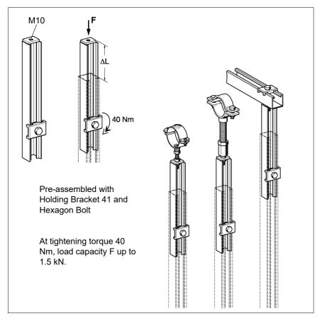
Continuous extension for Cantilever Brackets and Channels in series 41 (Channel height S 41 mm):
