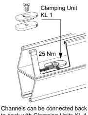
to back with Clamping Units KL 1 spaced at 500mm and at each channel end.
